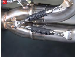
AG) Using the supplied hardware and spacer, attach the silencer to the original mounting point on the bike. Leave a little loose for now, you will fully tighten in a later step.
