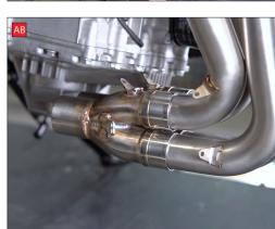
Y) Support the weight of the exhaust system, then remove the mounting bolt/nut.
