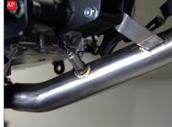
AO) Plug the lambda sensor into the extension cable and clip the cable back in place.
